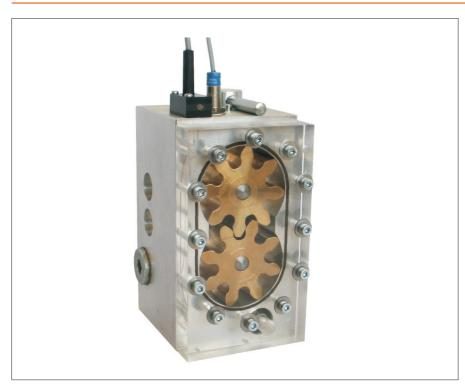
Volume flow meter with throttle- and bypass valve KUZ-L
