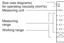
Within the working range the float with its ring marking can move.
